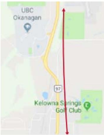
An extension of Acland Road to Bulman Road and to the Airport would provide a new continuous connection between the Airport, Acland Road and Rutland Road on the east side of Highway 97. It would improve network redundancy by providing a new Airport road connection, and it has been previously considered in other planning processes.
