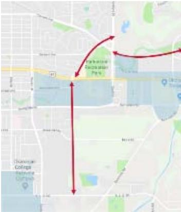
**Glenmore to Burtch Connection** - A connection between Glenmore Drive and Burtch Road exists via Bernard Avenue. This option would strengthen this connection and relieve pressure from Spall Road. It would need to be developed in conjunction with the redevelopment of the Apple Bowl site and future school site.
