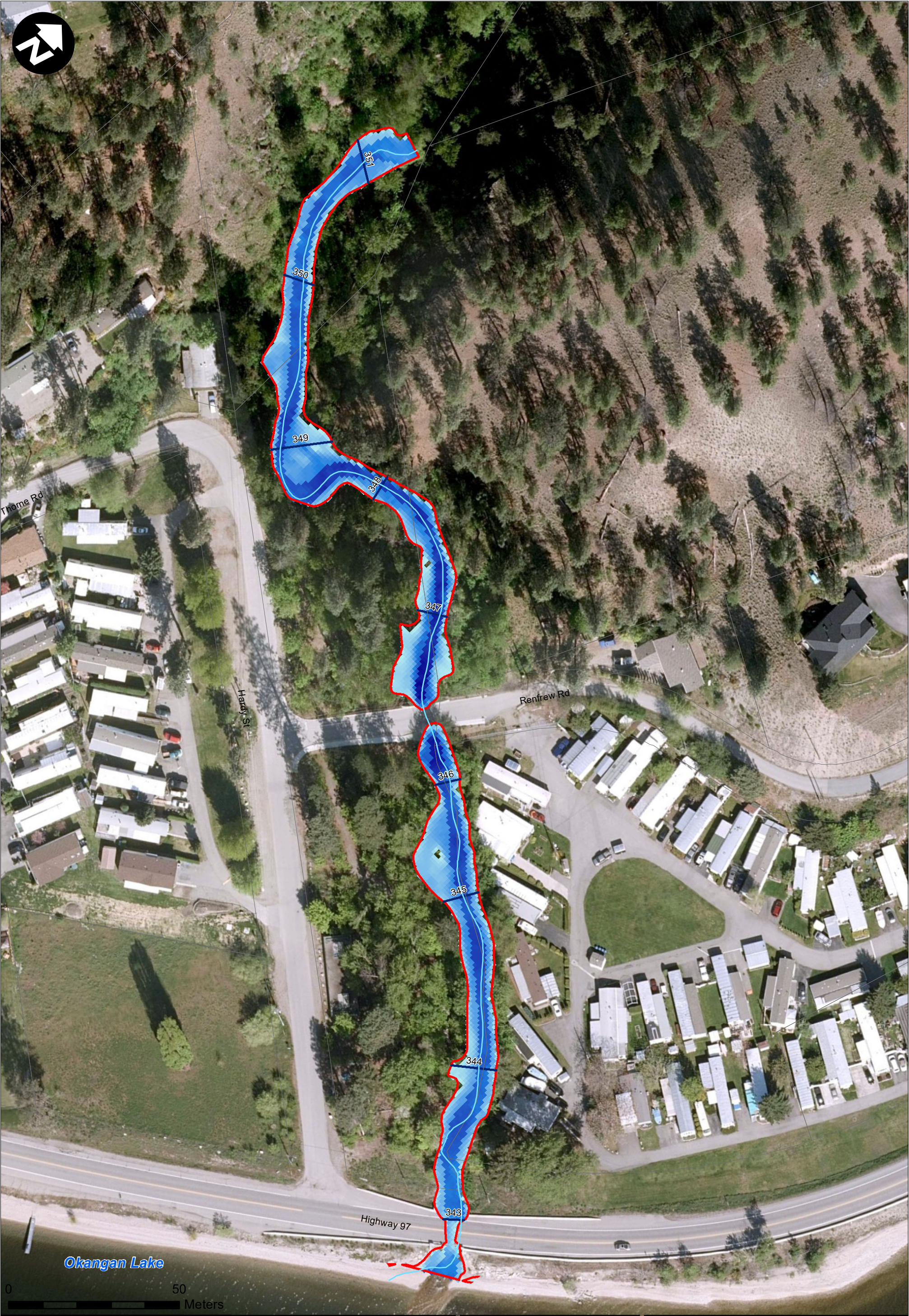
FIGURE 5-1: PEACHLAND CREEK REACH 1, 20-YEAR FLOOD EXTENTS RDCCO Peachland and Trepanier Creek Flood Mapping
