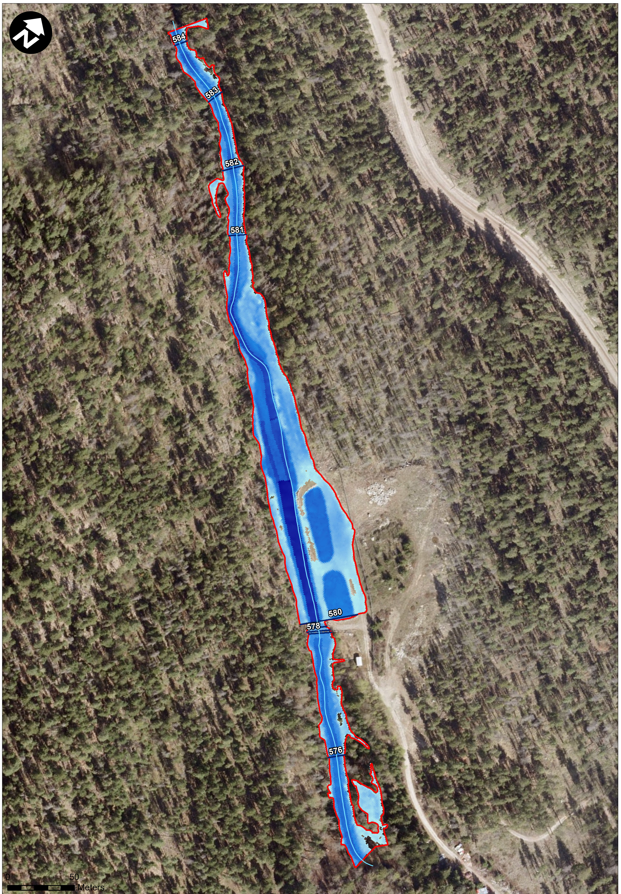
FIGURE 5-5: TREPANIER CREEK REACH 3, 20-YEAR FLOOD EXTENTS RD Peachland and Trepanier Creek Flood Mapping
