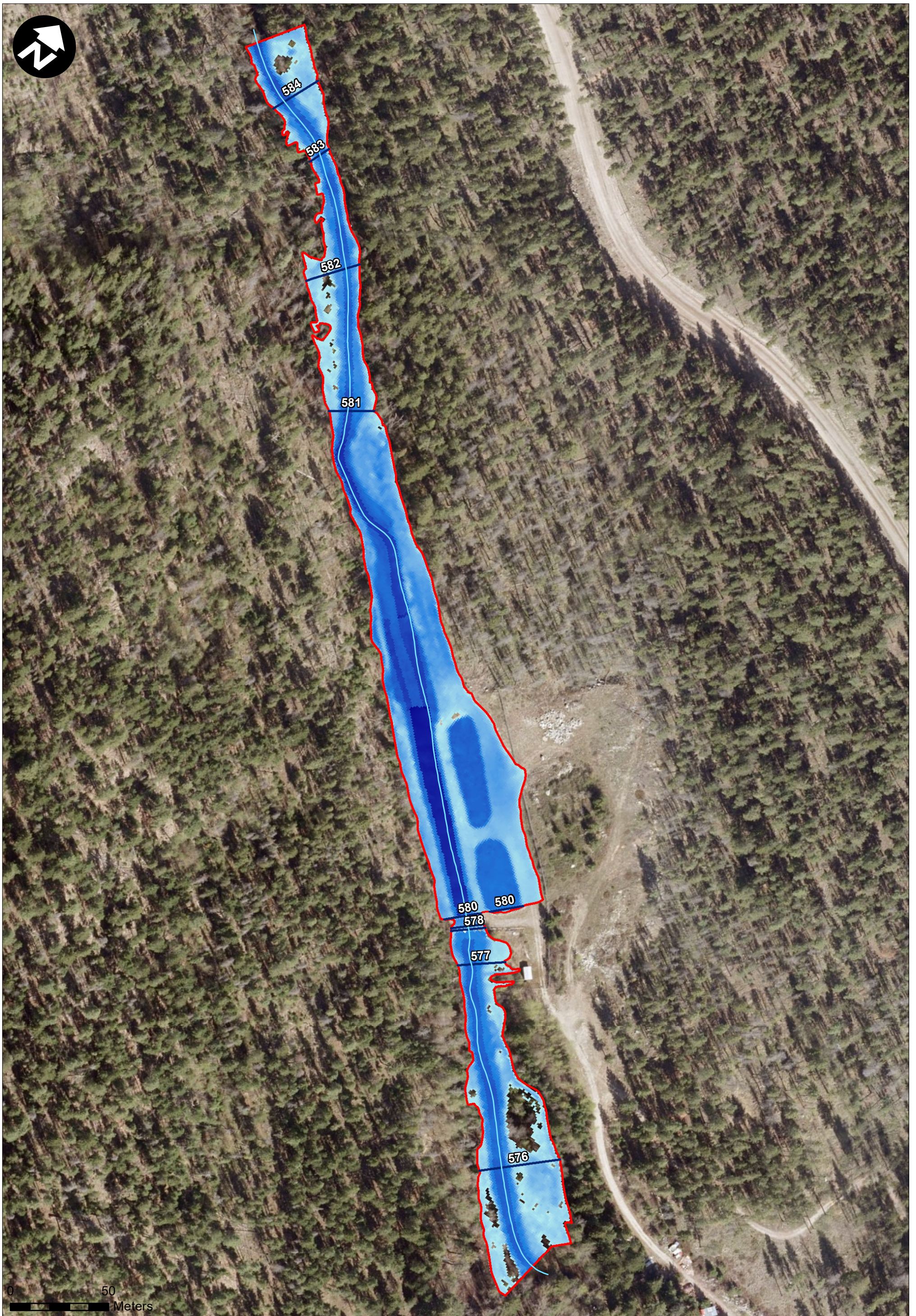
FIGURE 5-6: TREPANIER CREEK REACH 3, 200-YEAR FLOOD EXTENTS RD Peachland and Trepanier Creek Flood Mapping
