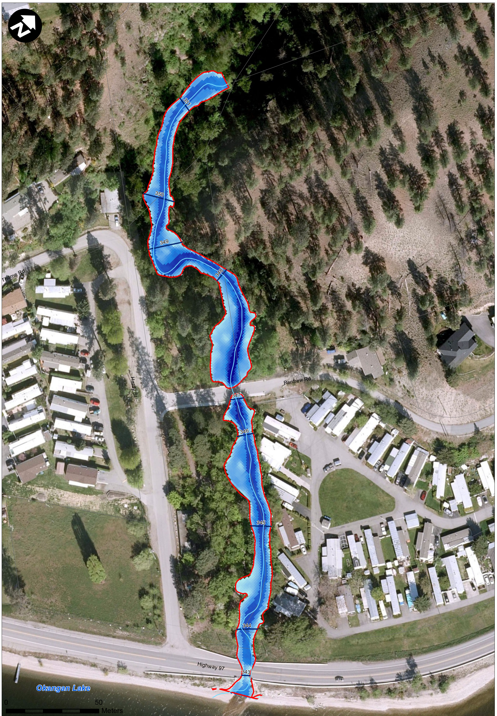
FIGURE 5-2: PEACHLAND CREEK REACH 1, 200-YEAR FLOOD EXTENTS RDCO Peachland and Trepanier Creek Flood Mapping
