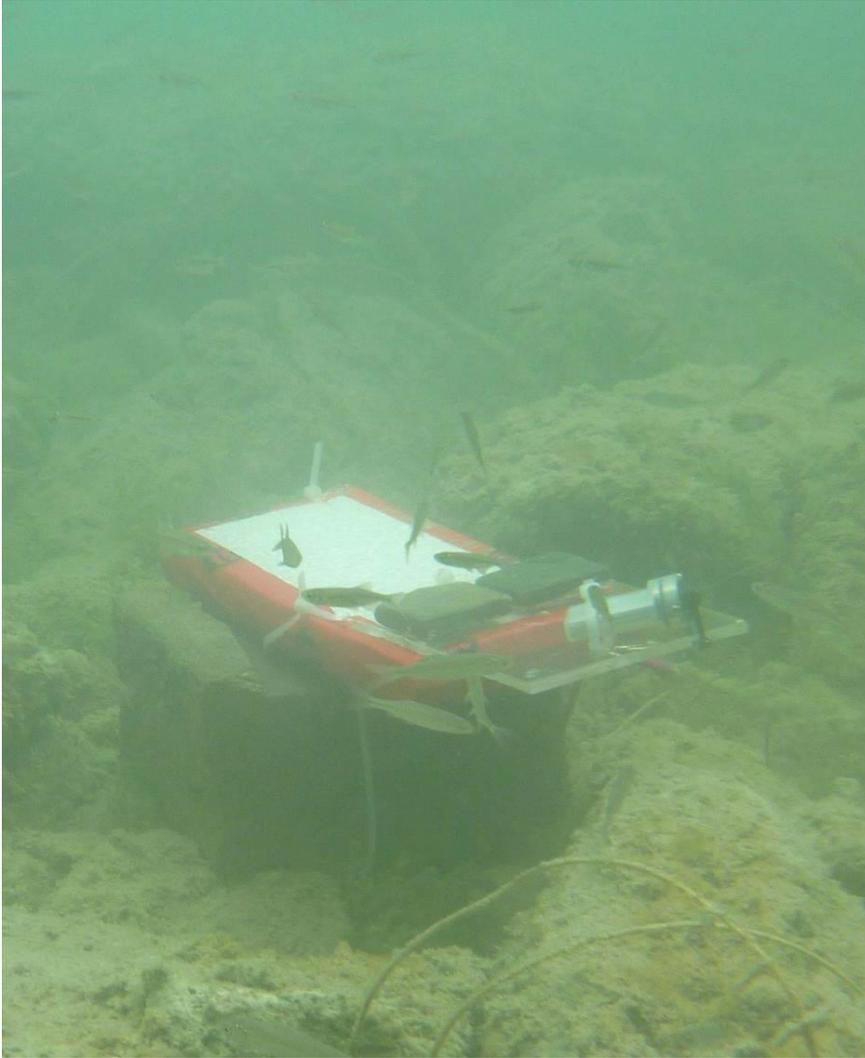
**Figure 3: Example of Periphyton sampler**
