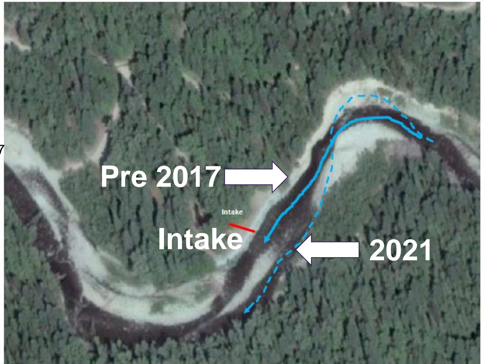
Figure 2 – Original flow path past intake in 2017 (solid blue line) and 2021 flow path (dashed blue line).
