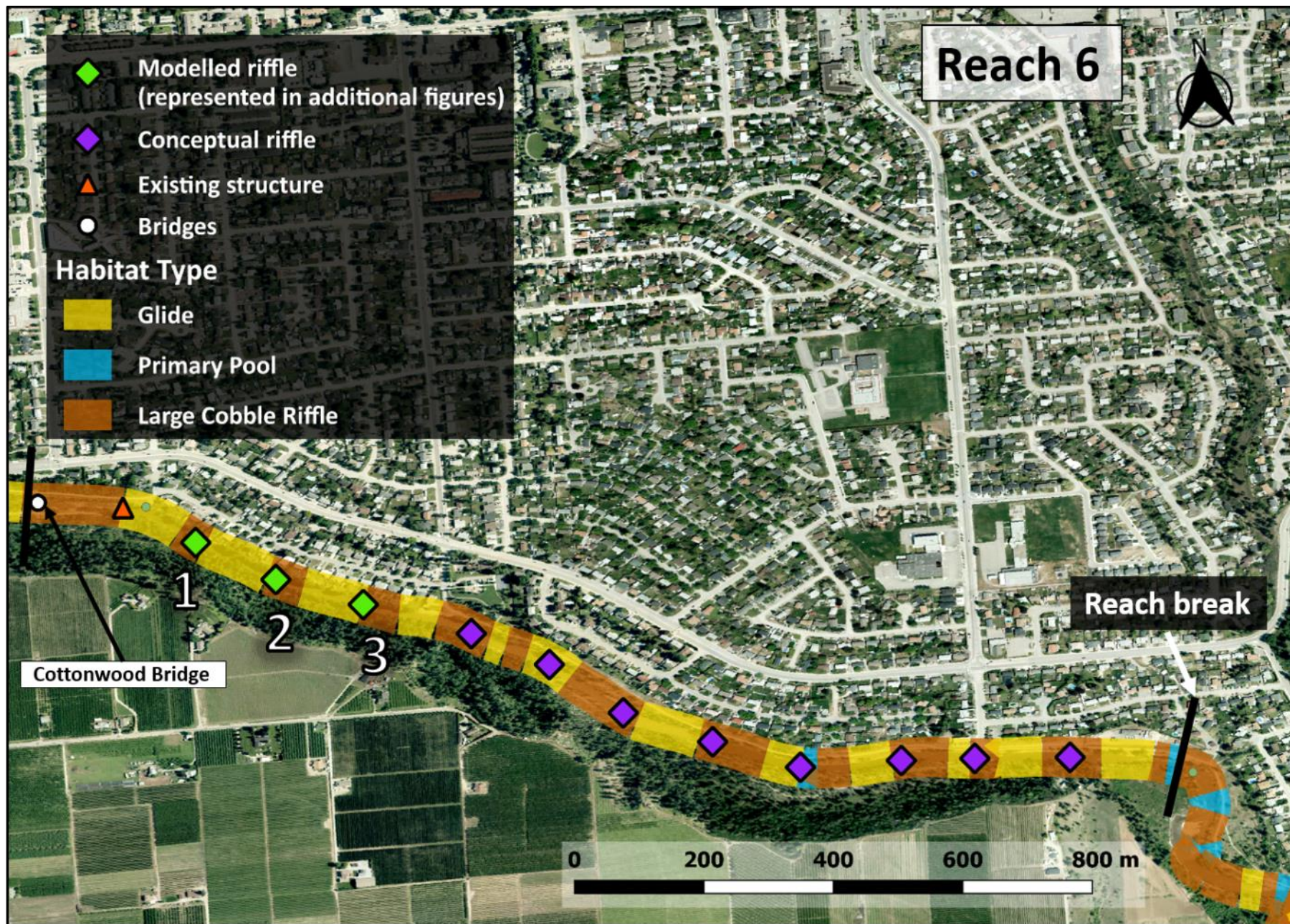
Figure 12: Reach-6 habitat conditions and restoration design recommendations
