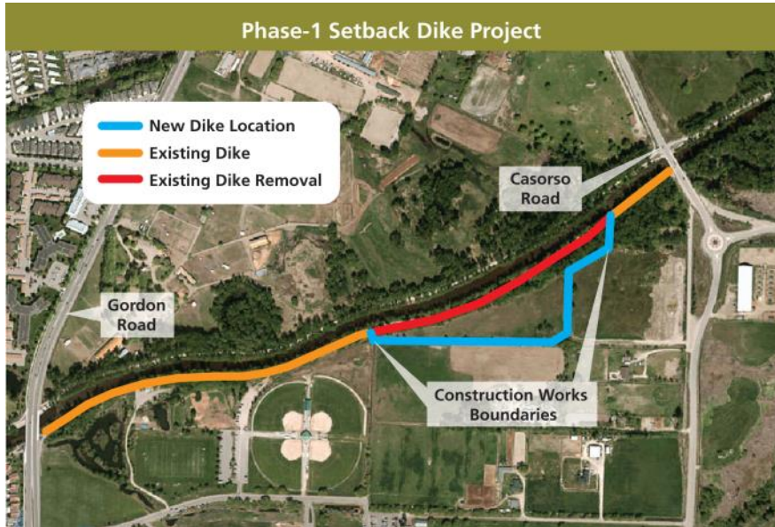
MCRI's first large-scale habitat restoration project re-naturalized floodplain function and re-established important fish habitat features within Mission Creek between Casorso Road and Gordon Drive.
