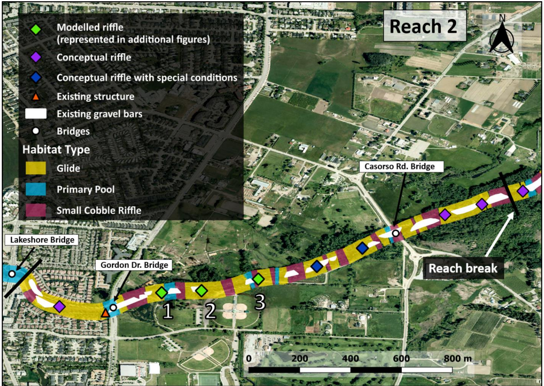
Figure 8: Reach-2 habitat conditions and restoration design recommendations
